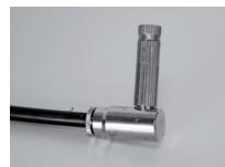
4. Screw the nozzles into the connectors
