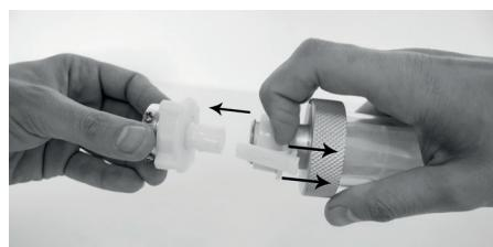
4. Connect the suction pipe to the machine in the lower connection.
